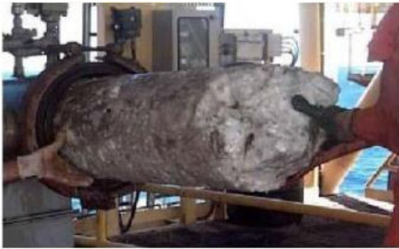
Figure 42: Hydrate formation in the natural gas pipeline [33]
